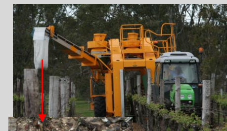
Figure 1. Head setup for snail removal
