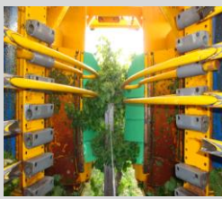
Figure 5. Head setup - 2 beater rods
